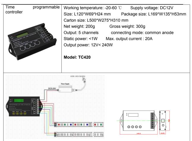
1. It can make the load output change over time, the customer may customize schedule mode they want through the upper PC. Then through the USB port to download required schedule to the controller
